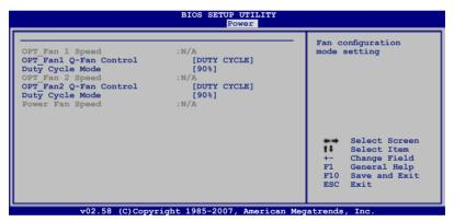
The onboard hardware monitor automatically detects the optional fan speed. If the fan is not connected to the motherboard, the field shows N/A.
